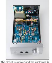
more rigid for better sound. The negative effects due to noise and vibrations are reduced.
